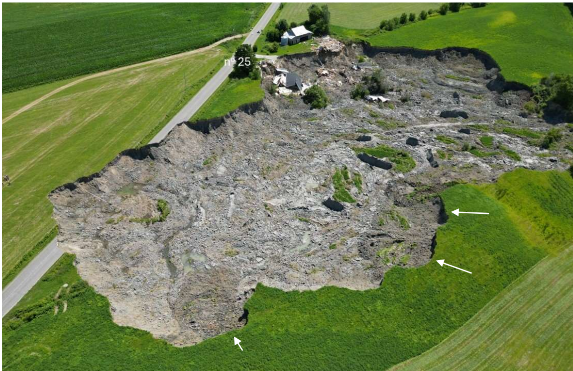
Figure 8: Aerial view of the landslide taken by drone on July 20, 2025. The photo shows the now-destroyed residence no. 25, as well as recent rotational failures (white arrows) around the scar. (Source: MTMD)
