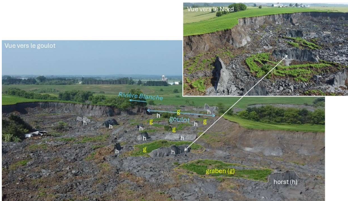
Figure 7: View of horsts (h) and grabens (g) inside the landslide scar. (Source: MTMD)
