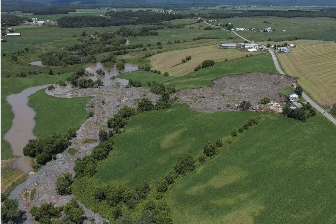
Figure 6: Overview of the landslide scar and part of the debris obstructing the Blanche River on July 16. Note the new channel the river has started to follow on the left. (Source: MTMD – DJI_20250718131933_0159)
