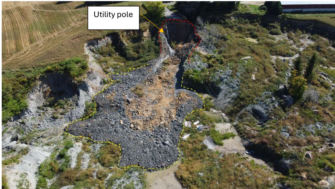
Figure 12 : Recent landslide (mid-September 2025) that toppled a utility pole. Note the significant remoulding of debris associated with this event.
