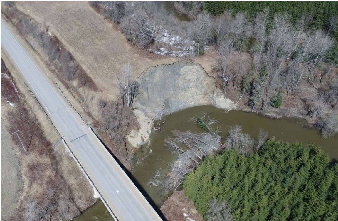
Figure 6 : Drone view of the April 2022 landslide along the Noire River, near the road and bridge on Saint-Philippe Road. (Source: MTMD – DGG)
