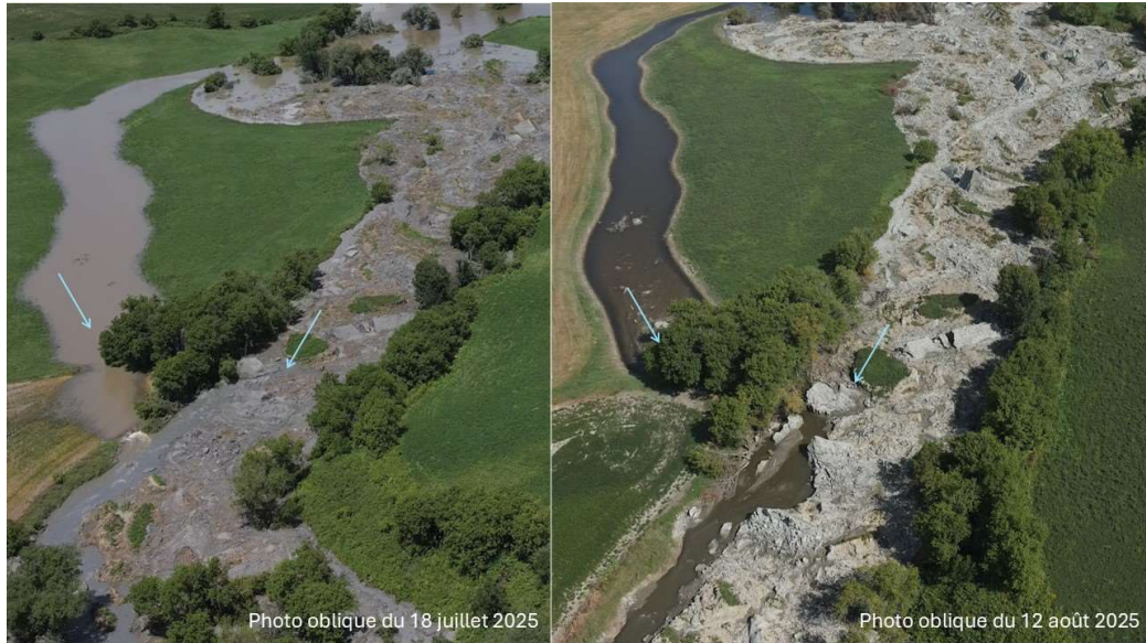
Figure 12: Drone photos at the confluence between the main Blanche River channel and an old branch now carrying the river's flow after the landslide. Arrows indicate flow direction. (Source: MTMD-DGG)
